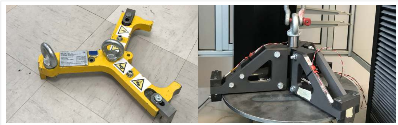
The original lifting tool (L) was machined out of solid steel and weighed 75% more than its 3D printed replacement (R).
