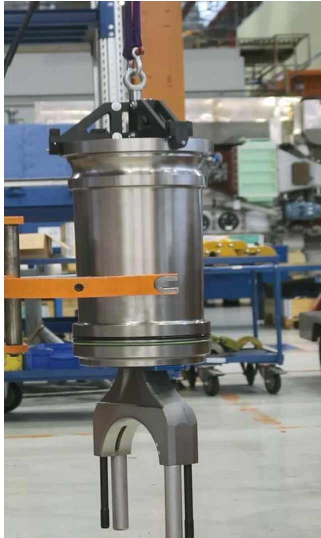
The tool is capable of lifting up to 960kg with a safety factor of four.
